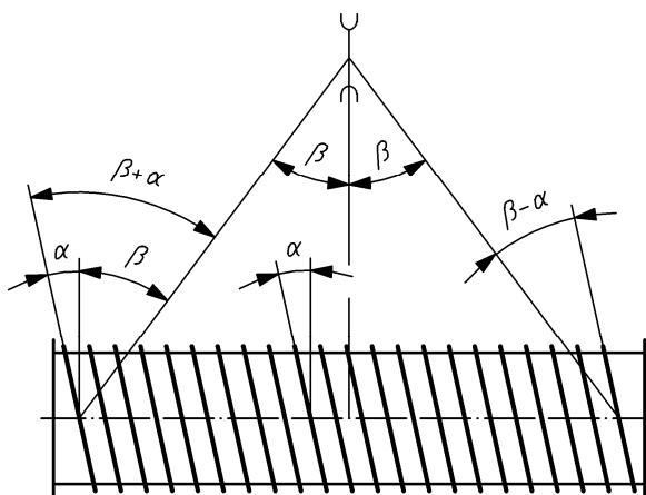
**Key** $\beta$  = fleet angle on the pulley $\beta - \alpha$  or  $\beta + \alpha$  = fleet angle on the drum $\alpha$  = angle of the grooves on the drum
