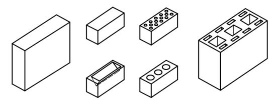
a) Group I Units which are solid or with  $\leq 25$  % by volume of formed vertical holes that may or may not pass right through the unit, or units with  $\leq 25$  % by volume of frogs in the bed faces
