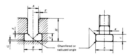
E, F and  $G: 45^{\circ}$ -chamfer height or radius
