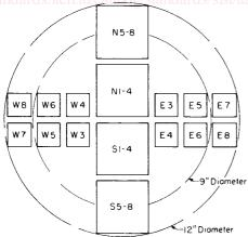
Note 1—Sticks cut from the *N-S* axis shall be  $2\frac{1}{2}$  by  $2\frac{1}{2}$  in. (60 by 60 mm) when green. Sticks cut from the *E-W* axis shall be  $1\frac{1}{4}$  by  $1\frac{1}{4}$  in. (30 by 30 mm) when green.
