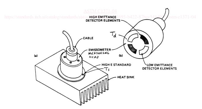
Note 1—(a) Emissometer measuring head on high-emittance standard during calibration, showing heat sink and cable to readout device. (b) Bottom view of emissometer measuring head showing high- and low-emittance detector elements. The diameter of the emissometer measuring head is about 50 mm and the detector elements are recessed about 3 mm into the measuring head.
