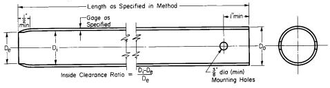
Note 1—Minimum of two mounting holes on opposite sides for D<sub>o</sub> smaller than 4 in. (101.6 mm).
