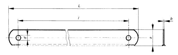
Blade length / is the distance between centres of pin holes. It is recommended that the centre of the pin hole be located on the centrelline of the blade.
