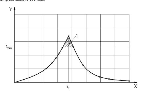
Figure 7 — Incorrect fuse selection
