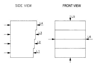
Note 1—Sound speed reference block manufactured of optical quality glass of high uniformity. The multiple sound propagation paths are marked L1 through L6.
