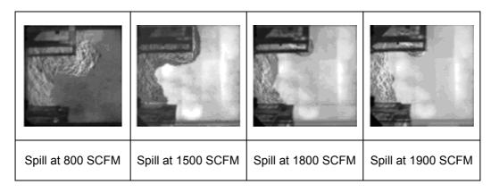
Figure 1 — Example of schlieren flow visualisation for gas charbroilers under a canopy hood
