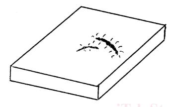
crazing—the cracking that occurs in fired glazes or other ceramic coatings as a result of tensile stresses, may also occur in the surface portion of uncoated (unglazed) whiteware bodies.
