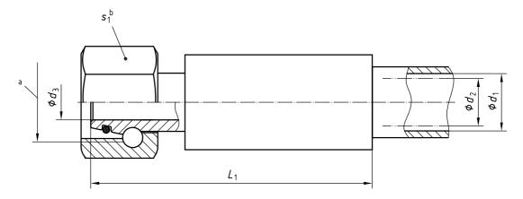
NOTE 1 A free length of tube should be left so that, in the case of an O-ring change, the nut can be moved behind the O-ring groove.
