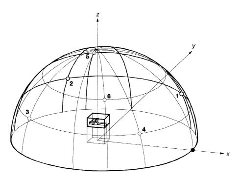
NOTE The microphone positions differ when determining the sound power level according to European Directive 2000/14/EC (see Annex D).
