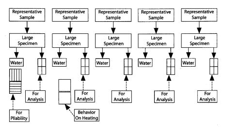
In Section 6, initial "Representative Samples" are selected (typically five per lot). These are full bundles or rolls. These are the samples used in Section 7.
