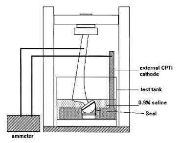
Note 1—The cathode sheet surrounds, but does not make contact with the device being tested. For Procedure A, the counter electrode is not utilized, and is substituted with a luggin probe and calomel electrode.
