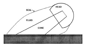
Note 1—For Method I, the fluid is contained within the sleeve. For Method II, the device should be submerged in an electrolyte while the contact area between the top of the head and the loading apparatus is not exposed to the fluid. A counter electrode is placed in the same bath.
