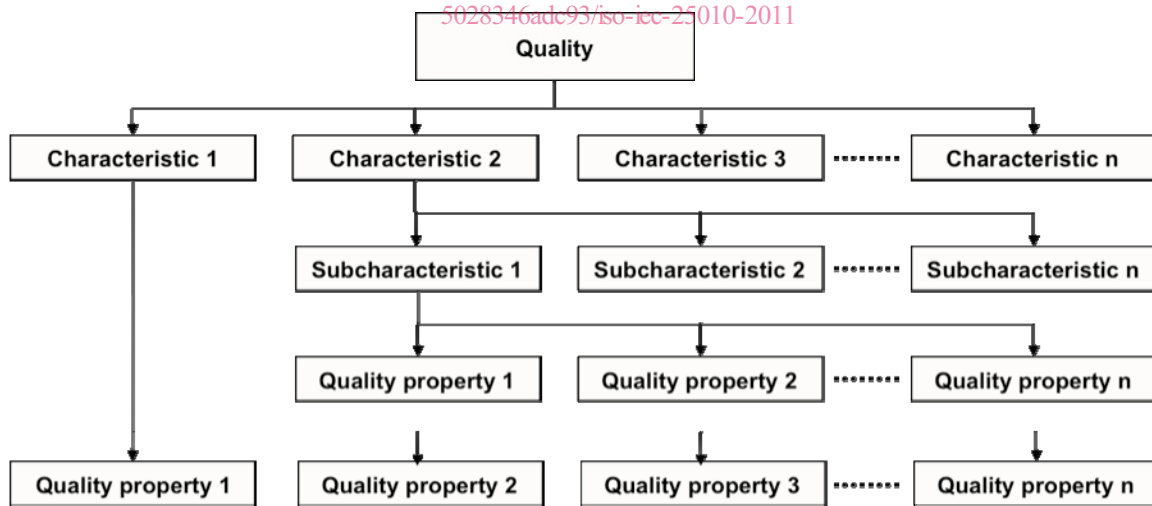
Figure 2 — Structure used for the quality models
