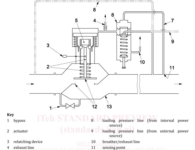
Figure 2 — Example N. 1 of an indirect acting gas shut-off device
