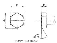
DIMENSIONS FOR TWIST OFF STRUCTURAL BOLT
