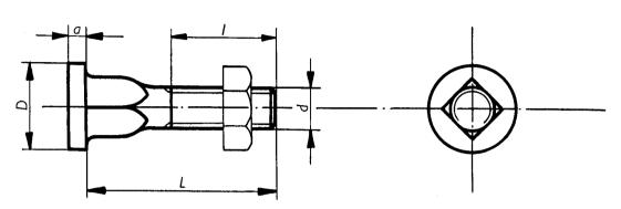
d = external diameter of screw thread = nominal diameter of deckbolt
