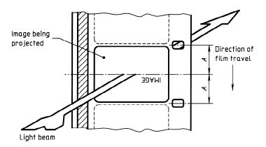
The film is shown as seen from the light source in the projector looking towards the projector lens.
