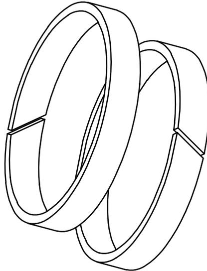
Figure 1 — Typical example of a rectangular-cut-section bearing ring
