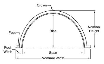
NOTE—The model chamber shown in this standard is intended only as a general illustration. Any chamber configuration is permitted, as long as it meets all the specified requirements of this standard. FIG. 1 Model Chamber 3.1.14 *web*—the element of a corrugated wall that connects a crest element to a valley element (see Fig. 2).
