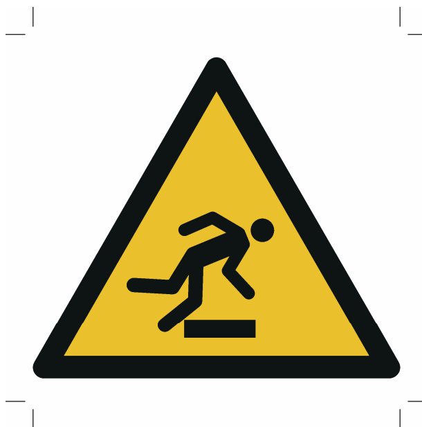
Figure 4 — Warning; Obstacles (ISO 7010, W007)
