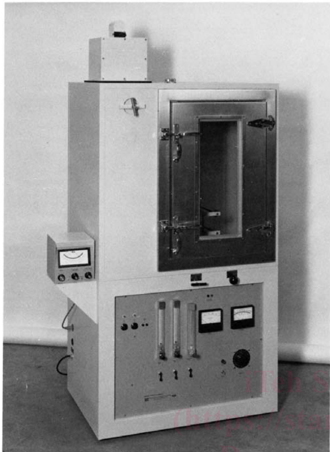
FIG. 1 Smoke Density Chamber
