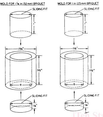
NOTE 1—Material: cold rolled or stainless steel. Dimensions a and b (inside diameters) are nominally 32 mm (1<sup>1</sup>/<sub>4</sub> in.) and 25 mm (1 in.). If an automatic polishing attachment is to be used, these dimensions should be specified to yield a briquet fitting snugly in the briquet holder.
