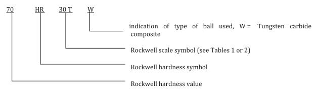
NOTE 1  $\,$  Previous versions of this part of ISO 6508 allowed the use of steel indenter balls, which required the suffix S.
