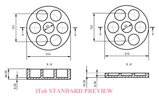
NOTE Adapt the dimensions of the holes according to the dimensions of the beakers available.
