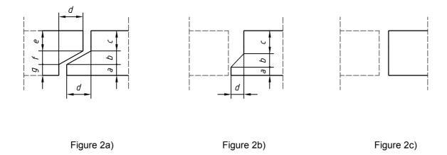
Figure 2 — Examples of box culvert joints
