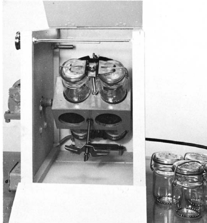
FIG. 1 Washing Machine, Heated Air Bath (Procedure B)
