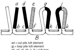
ab, cd, ef, gh, ij, jk = tuft legs cd, ef = cut pile tuft leg pair ij, jk = loop pile tuft leg pair, a loop B = one binding site
