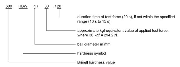
NOTE In former standards, in cases when a steel ball had been used, the Brinell hardness was denoted by HB or HBS.
