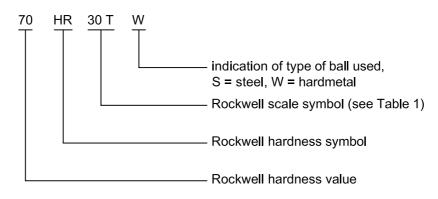
NOTE The numbers representing the test forces were originally based on units of kgf. For example, the test force of 30 kgf has been converted to 294,2 N.
