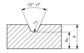
Radius  $r_N$  of notch base = 1 mm ± 0,05 mm b = specimen width (10 mm ± 0,2 mm)  $b_N$  = remaining width at notch base (8 mm ± 0,2 mm)
