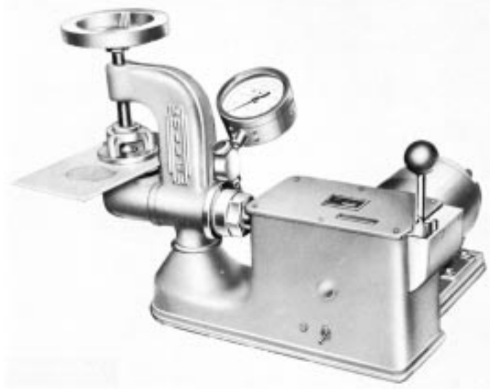
FIG. 1 Mullen Tester, Model A
