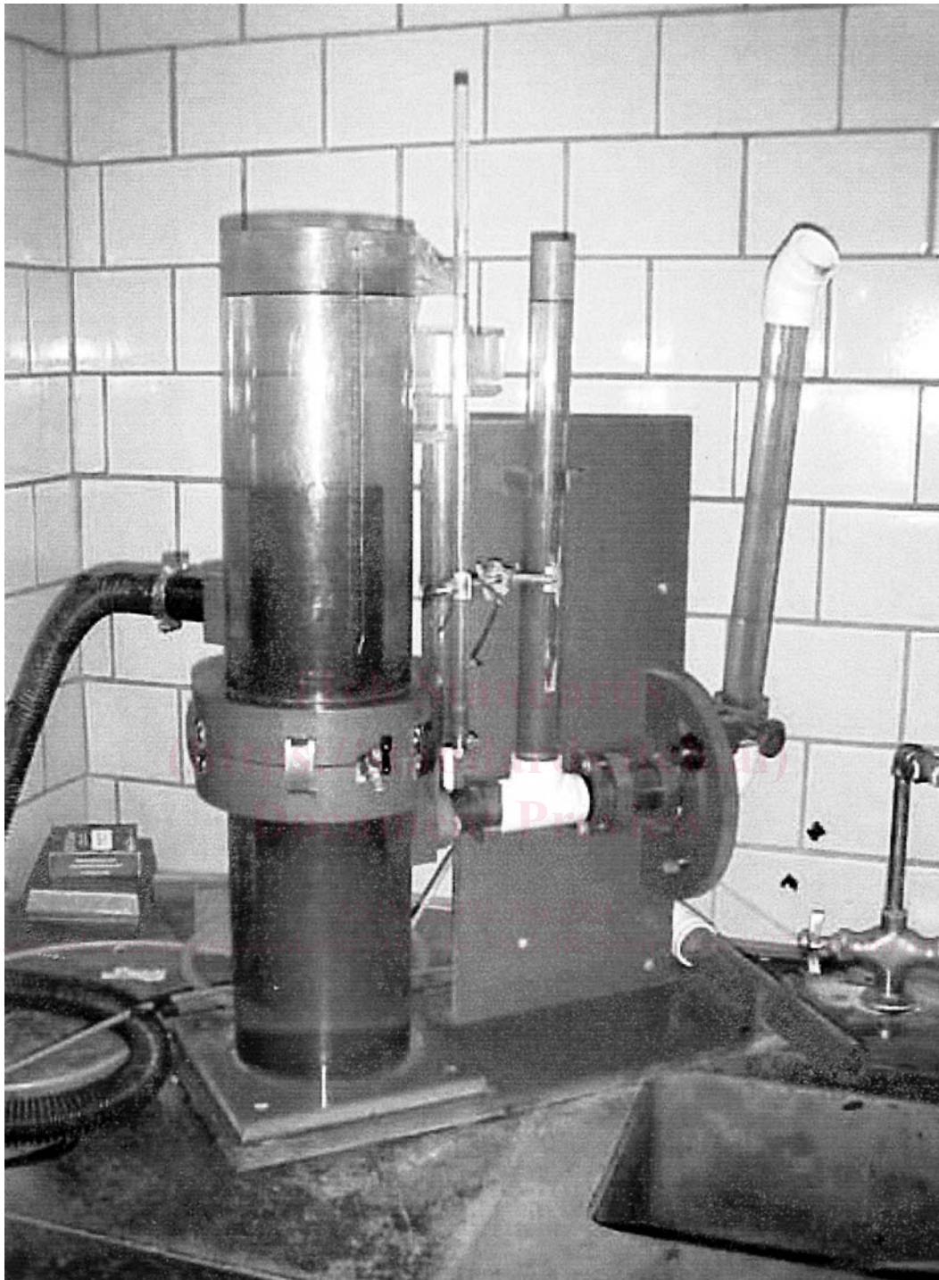
FIG. 1 Constant and Falling Head Permeability Apparatus
