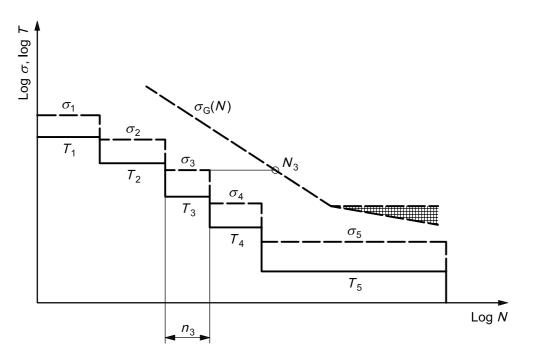
NOTE 1 The representation of the cumulative stress spectrum entirely below the S-N curve does not imply that the part will survive the total accumulative number of stress cycles. This information can be gained from a presentation as shown in Figure 3.
