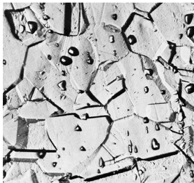
FIG. 1 Step Structure (500×) (Steps between grains, no ditches at grain boundaries)
