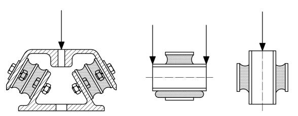
NOTE 1 When a resilient support has no parallel flanges, an auxiliary fixture is included as part of the test element to arrange for parallel flanges.
