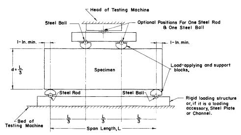
Note 1—This apparatus may be used inverted. If the testing machine applies a force through a spherically sealed head, the center pivot may be omitted, provided one load-applying block pivots on a rod and the other on a ball.
