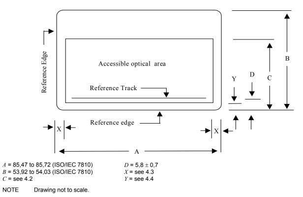
Figure 1 — Dimensions and location of the accessible optical area
