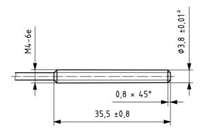
The gauge shall be of hardened steel.
