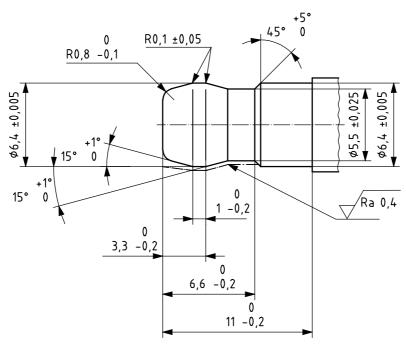
The gauge shall be of hardened steel.h STANDARD
