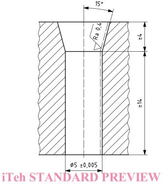
The gauge shall be of hardened steel (Standards.iteh.ai)
