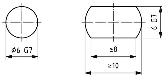
NOTE In  $\varnothing 6\ G7$ ,  $\varnothing$  indicates diameter, the 6 represents 6 mm, and G7 is a "class of fit" tolerance which is a sliding fit for a hole.
