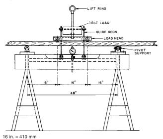
Note 1—This device is used for assessment of E in third-point, flat-wise bending on a span-to-depth ratio of 32 for  $1\frac{1}{2}$ -in. (38-mm) thick lumber.
