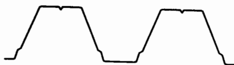
Figure 4 – Part of typical trapezoidal profile with stiffened crown and web
