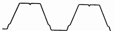
Figure 4 — Part of typical trapezoidal profile with stiffened crown and web
