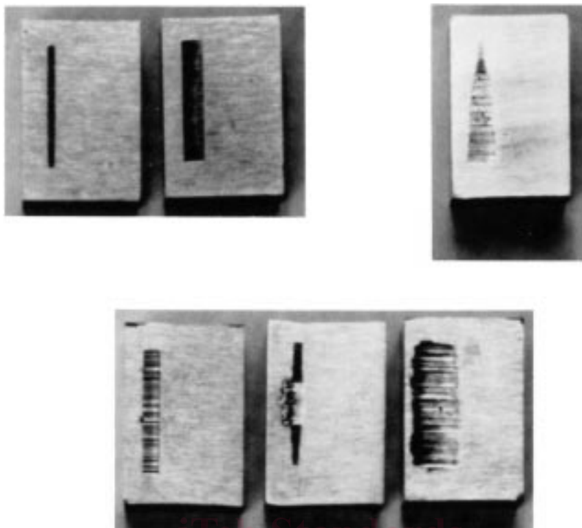
FIG. 1 Test Blocks Showing Various Types of Scar
