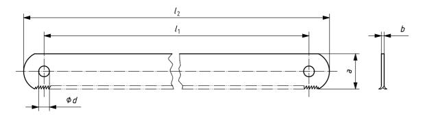
NOTE The shape of the end blade is left to the manufacturer's discretion.
