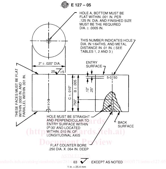
FIG. 1 Ultrasonic Standard Reference Block
