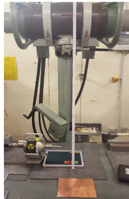
b) Photograph of measurement assembly with 420 kV tube, SDD = 1 m
