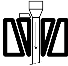
Figure 3 — Slip-type elevator with slips and setting ring
